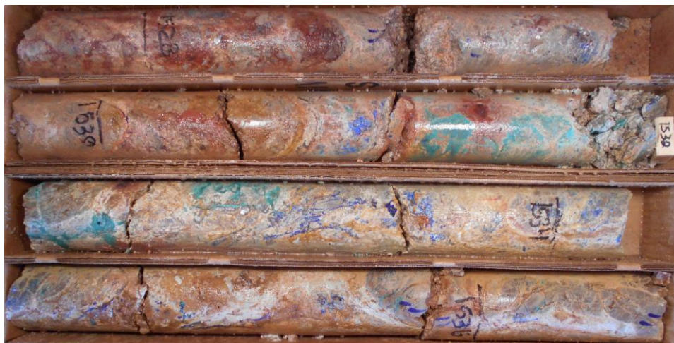
DDH VD14-04 6.57% AsCu 466.50m – 468.05m Malachite, azurite and chrysocolla
