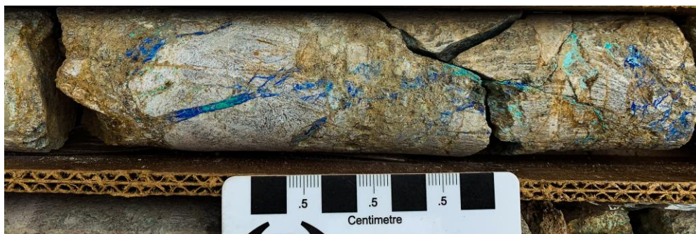
DDH M-3 294.5m Malachite, azurite and chrysocolla in fractured Pinal Schist
