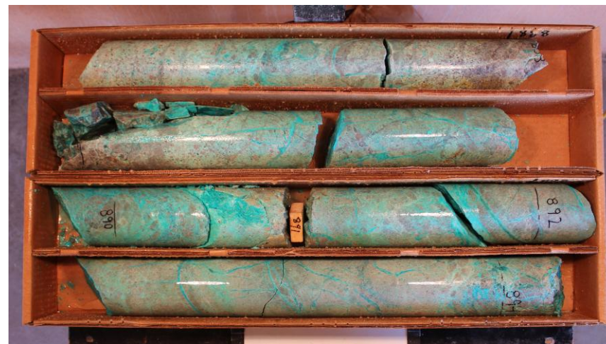
DDH VD14-06 3.29% AsCu 270.05m – 272.58m Malachite and chrysocolla in Pinal Schist
