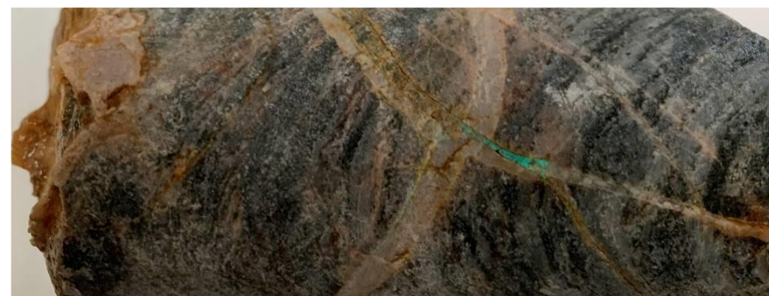
DDH OXY-47A 354.3m Quartz - Malachite vein in Pinal Schist
