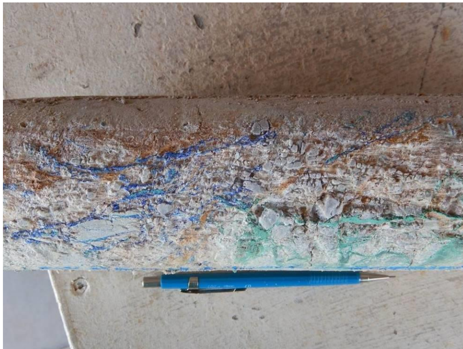
Plate 7-2 Brecciated Pinal Schist re-cemented in part by azurite and malachite, Drillhole VD-14-04 at 473.3m [the linear alignment of the mineralized structure suggest mineralized fracture]
