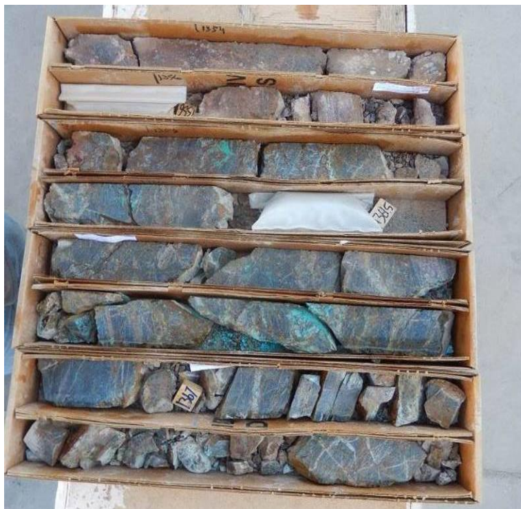
Plate 7-7 Malachite, azurite and chrysocolla in fractured to brecciated Pinal Schist, 412.46 – 417.67m, Drillhole VD-14-0
