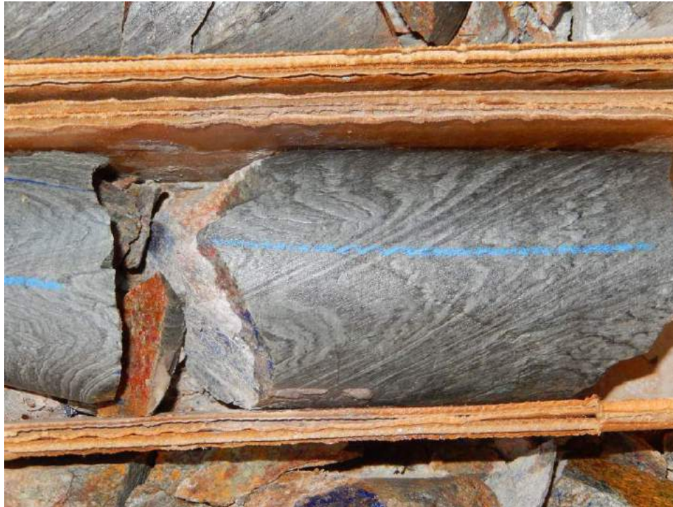
Plate 7-1 Chevron-folded Pinal Schist, Drillhole VD-14-05 at 439.7m
