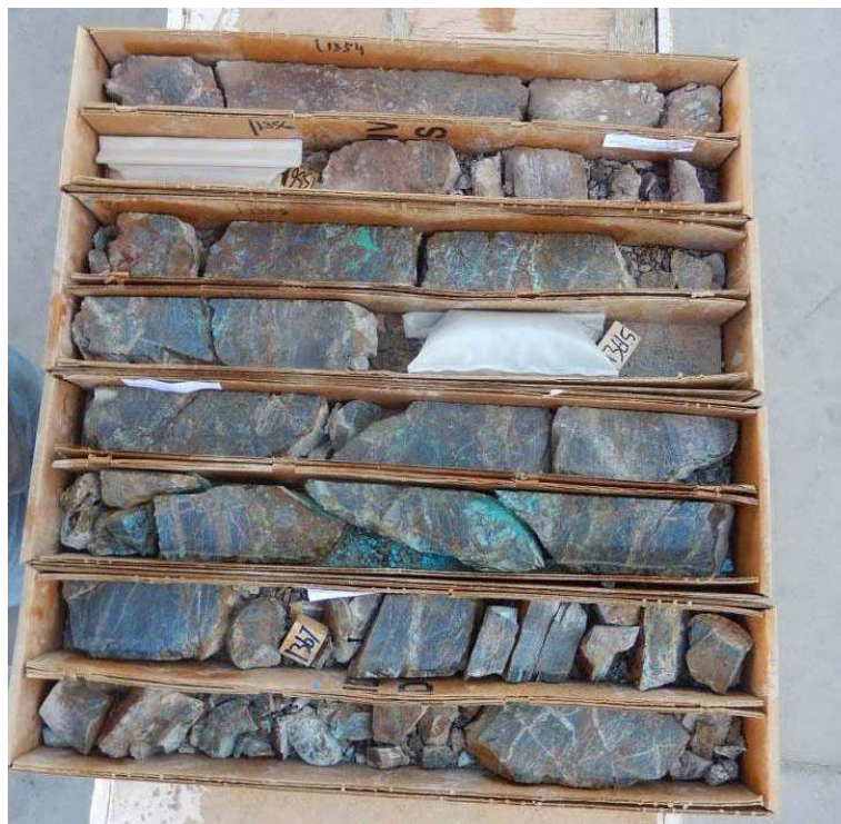
Plate 7-5 Malachite, Azurite and Chrysocolla in Fractured to Brecciated Pinal Schist, 412.46 – 417.67m in Drillhole VD-14-03
