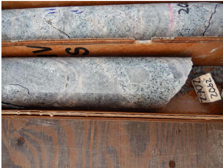
Plate 7-4 Schultze Granite, Drillhole VD-14-01 at 628.4m Showing Porphyritic Biotite Granodiorite with one zoned K-spar Megacryst
