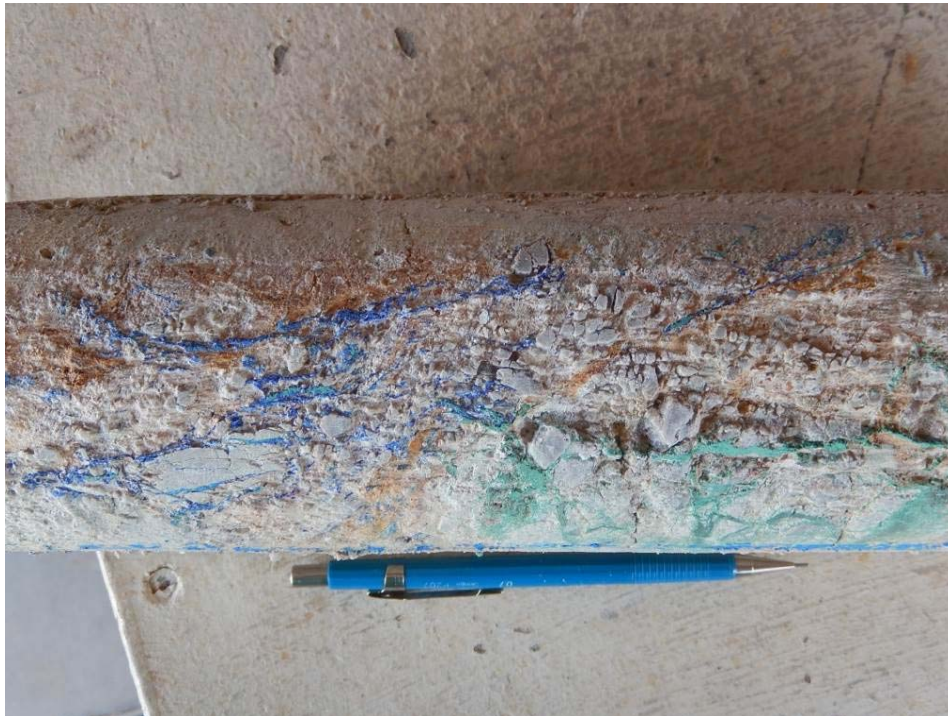
Plate 7-2 Brecciated Pinal Schist Re-cemented in Part by Azurite and Malachite, Drillhole VD-14-04 at 473.3m
