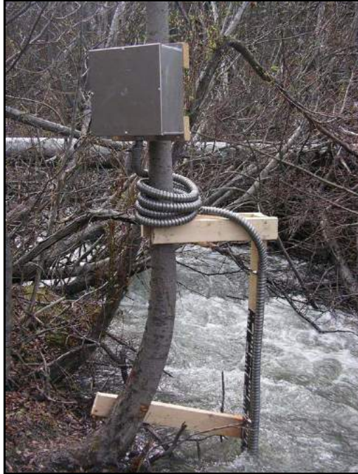
Plate 3.1-1. Sctr-1 hydrometric station showing staff gauge, data logger (in aluminium box) and pressure transducer (in aluminum conduit).
