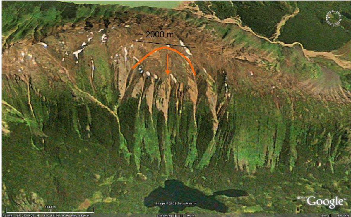
Figure 7.4 Tailing Storage Facility Sagged Slope Feature
