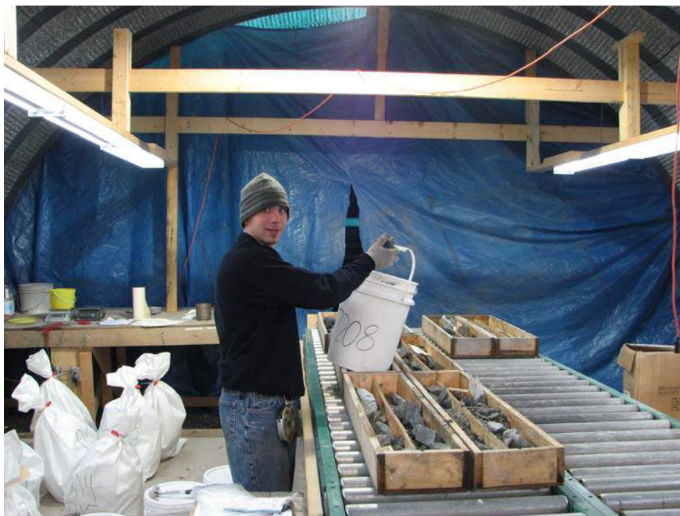
Figure 11-2: Sampling of PQ-core in quanset hut. Note roller system for moving heavy core boxes.
